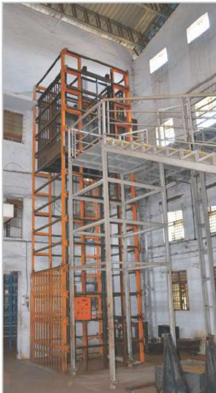
PLATFORM - 1500 X 2500 mm CAPACITY - 2000 Kg. LIFT - 5000 mm
