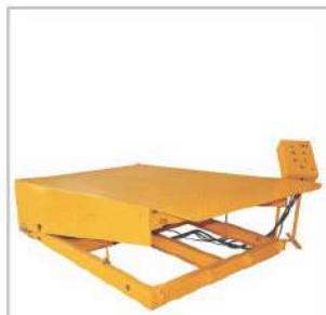
DOCK LEVELER IN MIDDLE POSITION (HT VARIABLE)
